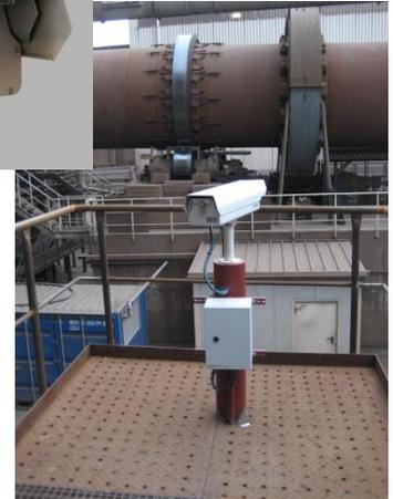
Infrared-Camera with Protective Housing installed in front of rotary kiln.
