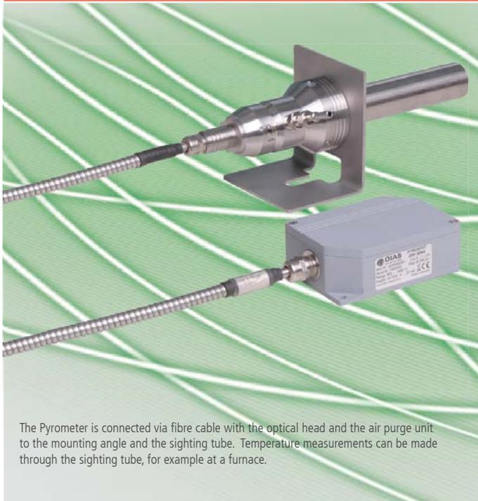
The Pyrometer is connected via fibre cable with the optical head and the air purge unit to the mounting angle and the sighting tube. Temperature measurements can be made through the sighting tube, for example at a furnace.
