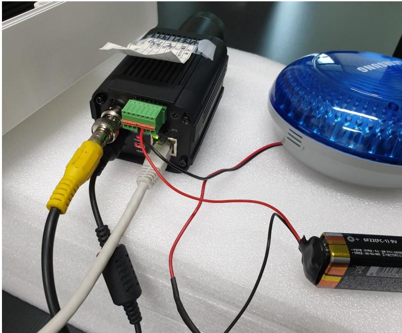
User must provide power to warning lamp separately or other device which will be operated when camera outputs alarm signal, as shown in the picture on the left.
