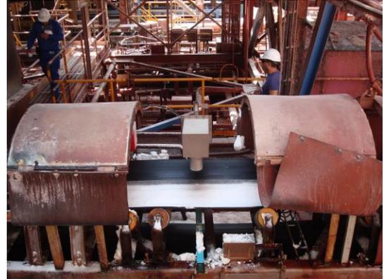
Measuring and controlling moisture can reduce transportation costs due to shipping excess water. Additionally, moisture control stops products from freezing during shipping and transportation.
