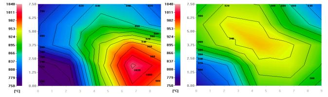
2D-temperature distribution of flue gas, waste incinerator, fixed bed.
