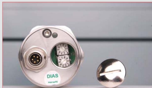
Emissivity can be adjusted directly at the device
