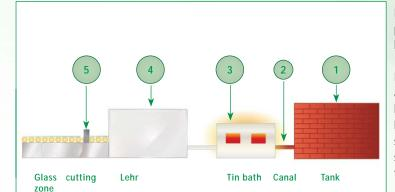
Different pyrometer models are used in the industrial floatglass production as the temperature of molten glass as well as solid glass have to be determined.
